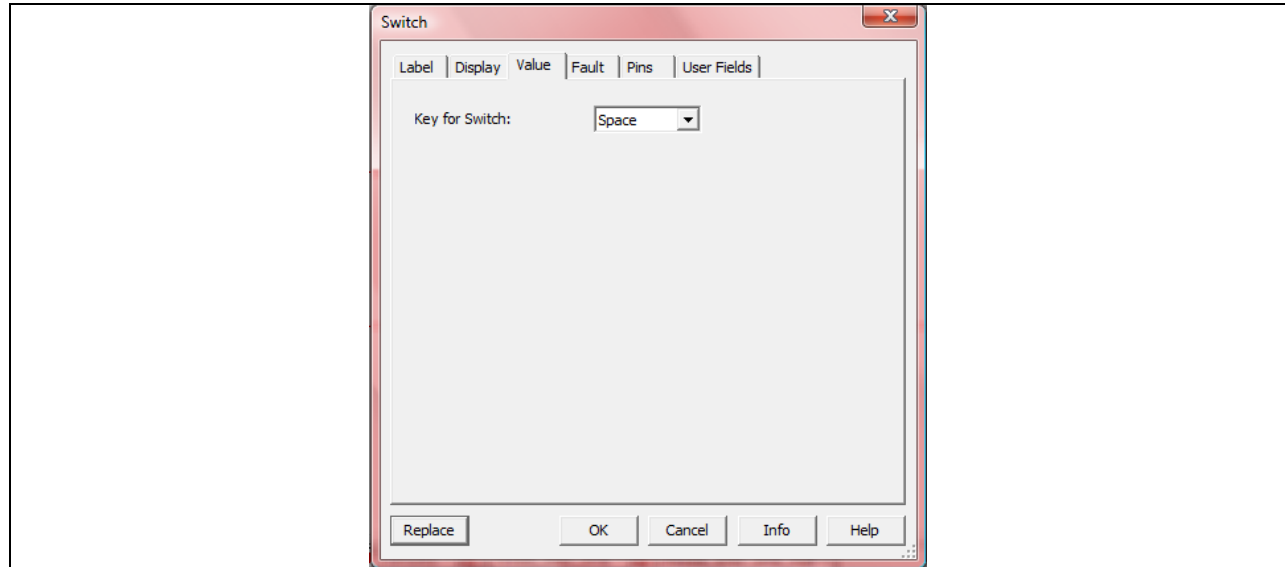
Figure 2.1.10 The Properties window for one of the SPDT switches in the schematic. By default the Value tab should be up front when the window opens. Clicking on the different tabs will allow access to different properties and characteristics of the switch.
