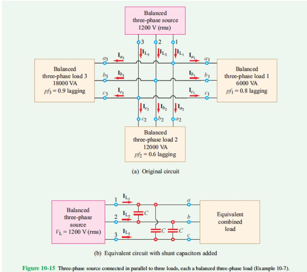
**Figure 10-15** Three-phase source connected in parallel to three loads, each a balanced three-phase load (Example 10-7).
