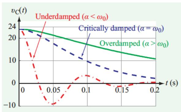
The underdamped response includes an oscillatory component.
